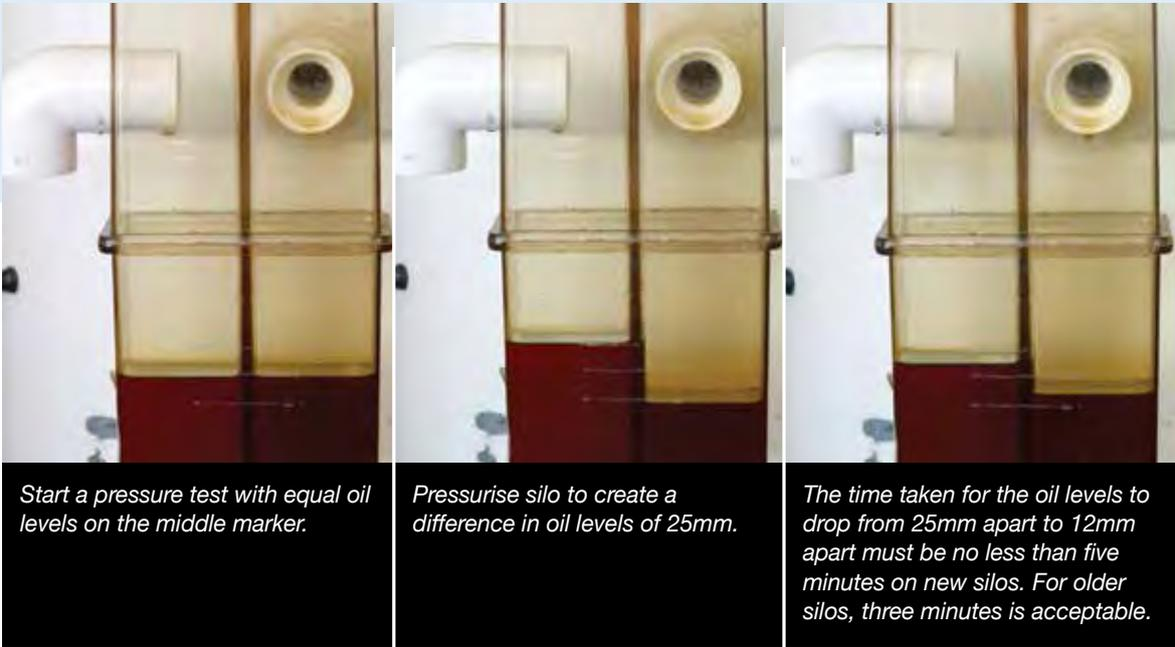
*Start a pressure test with equal oil levels on the middle marker.*
