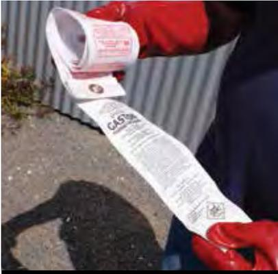
*In the bag: Phosphine in bag chains removes the risk of residue being spilt, but at least 1% of residue will not evolve until it comes into contact with moisture so a respirator and PPE are also required to remove it from the silo.*
