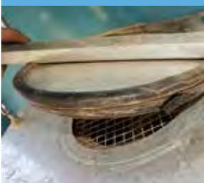
Before performing a pressure test, check seals around the lid, access hatch, hopper or boot and make sure the aeration fan seal is in a sound condition. Make sure all latches on lids and seal plates are locked down firmly.
