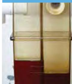
If fitted with an aeration fan, pressurise the silo by turning the fan on for a few seconds until the oil levels are more than 25mm apart. Then quickly turn the fan off and seal the fan inlet. This job is easier with two people — one to operate the fan and the other to watch the oil gauge.
