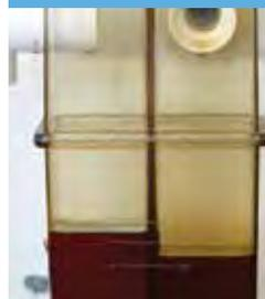
If oil levels are further apart than 25mm, wait until the pressure drops and the oil levels reach a distance of 25mm. The time taken for the oil to drop from 25mm to 12mm apart must be no less than five minutes on new silos. For older silos three minutes is acceptable.
