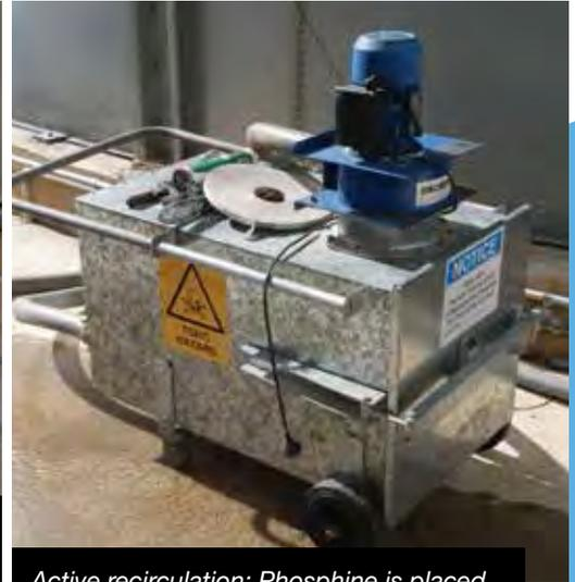
*Active recirculation: Phosphine is placed in the fumigation box and recirculated through the gas-tight silo.*
